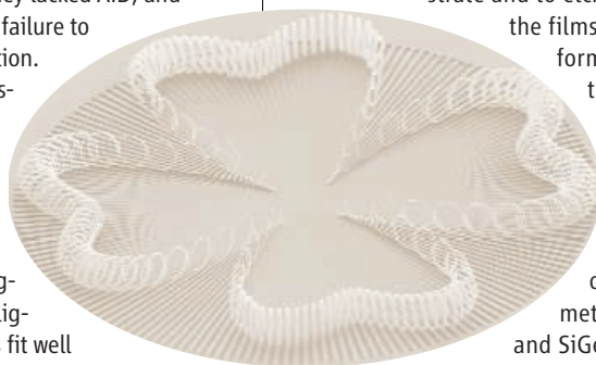
Scanning electron micrograph of Si/Cr bilayers; the similarity of coiling illustrates the dominant effect of the Cr layer over substrate direction.
